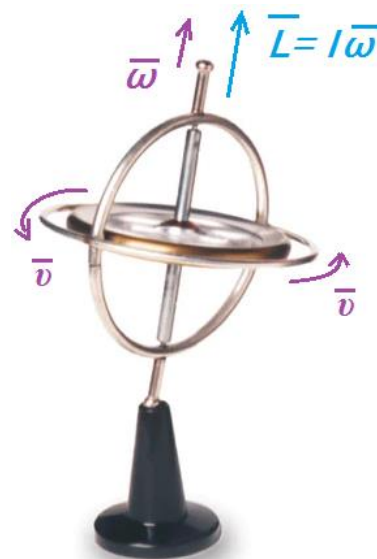
Figure 2. The law of conservation of angular momentum in a gyroscope
