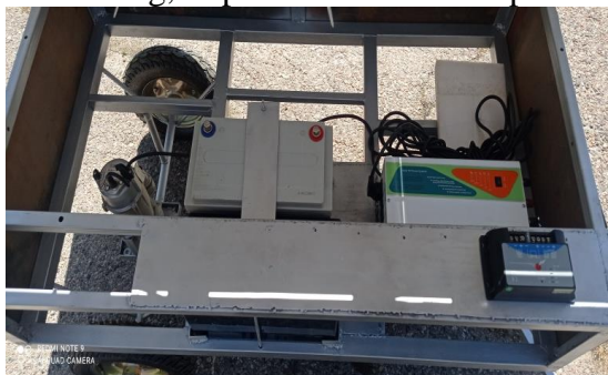
Figure 2. a - Arrangement of equipment inside the platform of the mobile photovoltaic device. b The assembled state of the mobile photovoltaic device
