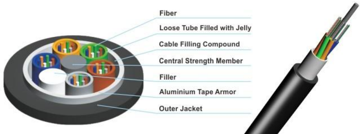
Figure 2: Reinforced optical fiber
