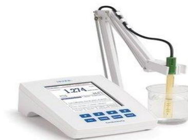
Figure 2. "HANNA" HI 5321 brand conductometer
